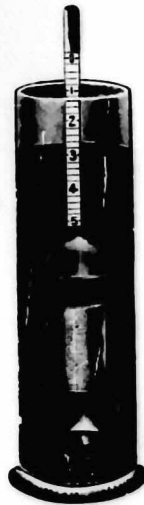
No. 6. Silver Solution Actinometer. Jar and Actinometer put in a wooden case.
