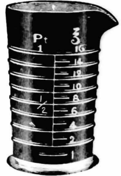
No. 25. Measuring Glass. Single American Scale. Pressed Lines and Figures.
